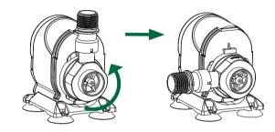
Remove impellor from the pump motor. Wash parts with fresh water carefully.
