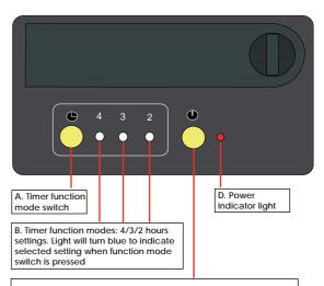
C. ON/OFF switch for continual use without timer function. This will run the feature until the battery power runs out.
